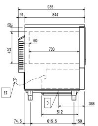
Drain Electrical inlet (power)
